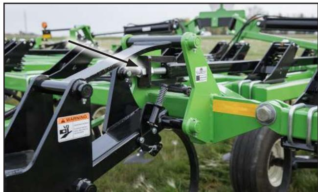
Fig. 62 Front to Rear Wheel Lift Connecting Arm
