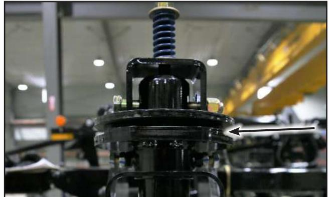
Fig. 64 Brake caster assembly
