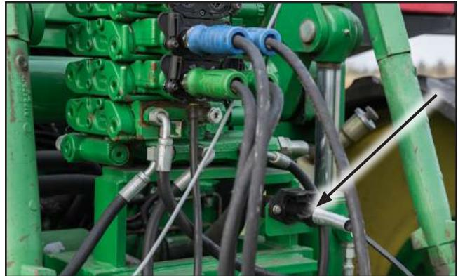
Fig. 11 Wiring Harness
