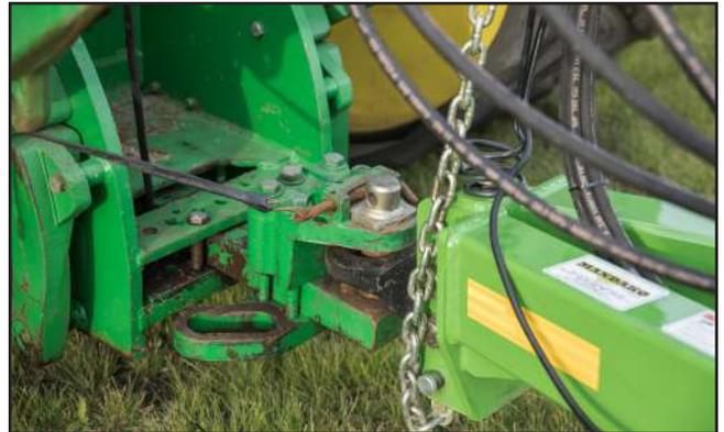
Fig. 7 Drawbar Pin and Retainer
