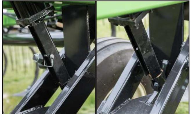
Fig. 21 Cylinder Stop: Pinned/Pin Removed
