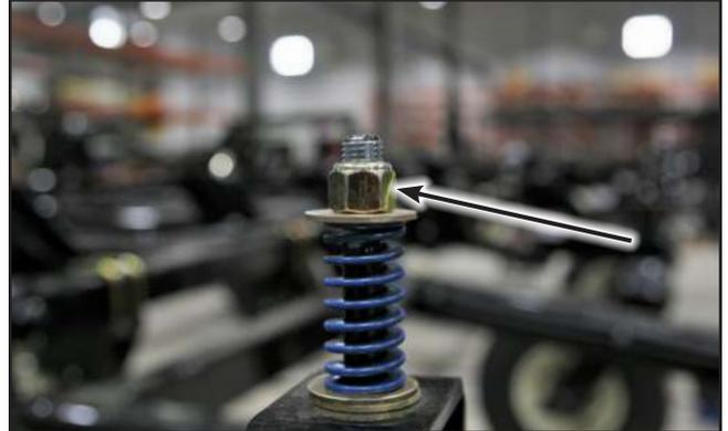
Fig. 63 Caster adjustment nut
