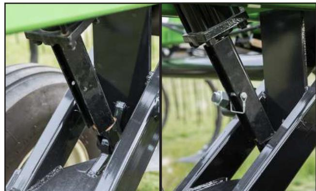
Fig. 47 Cylinder Stop: Pin Removed/Pinned
