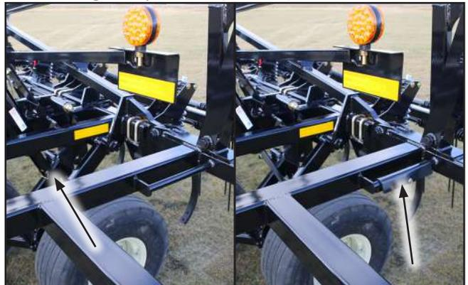
Fig. 22 Cylinder Stop: Installed/Removed and Stored
