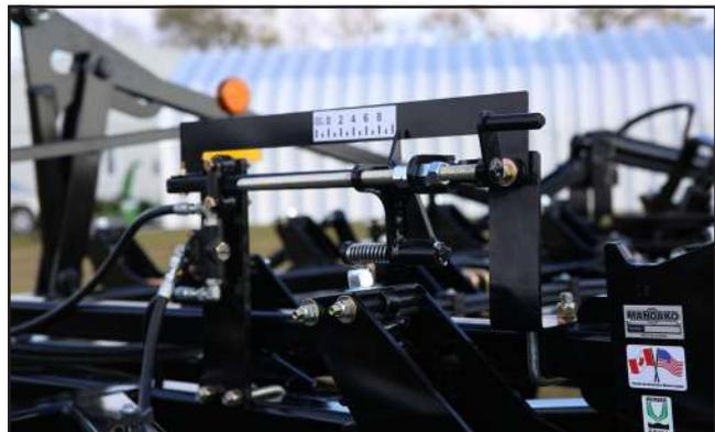
Fig. 41 Single Point Depth Control
