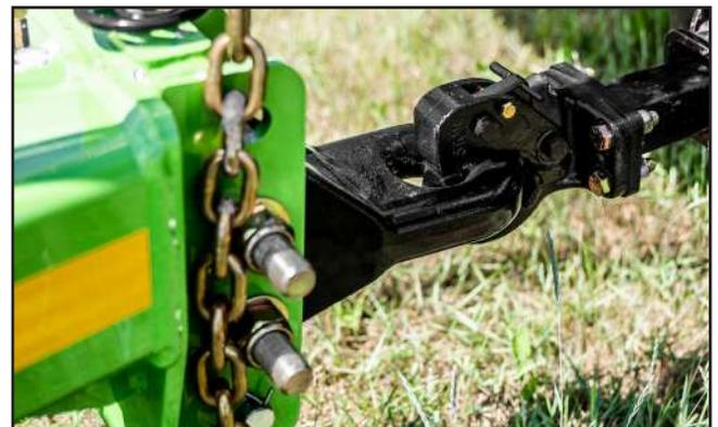
Fig. 16 Lock Pin/Bolt
