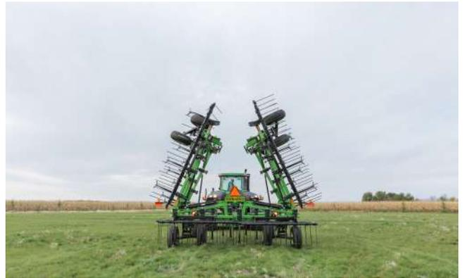
Fig. 50 Lift Wings: Lifted
