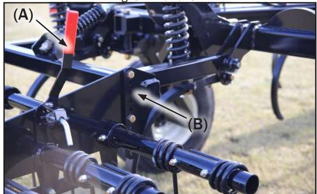
Fig. 33 Harrow Angle/Bolt Holes
