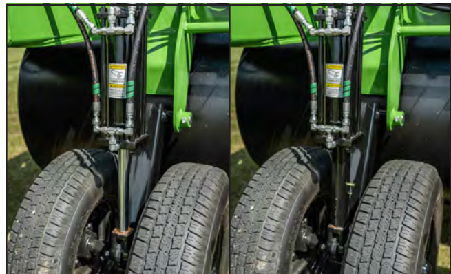
Fig. 55 Center Section Cylinder Stop: Removed/Installed
