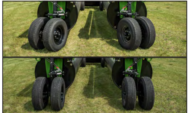
Fig. 58 Steerable Wheels: Turned/Straight
