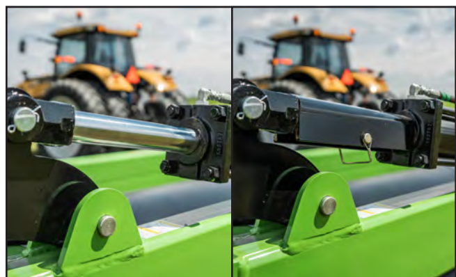
Fig. 56 Wing Section Cylinder Stop: Removed/Installed
