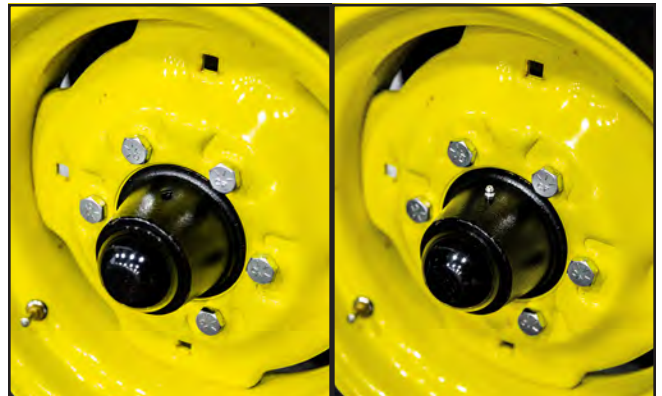
Fig. 71 Wheel Hubs: Plug/Zerk
