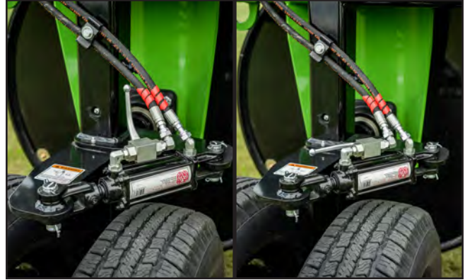
Fig. 47 Steering Circuit Hydraulic Ball Valves: Closed/Open
