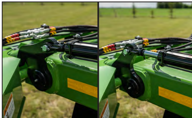
Fig. 51 Wing Lock Hooks: Disengaged/Engaged
