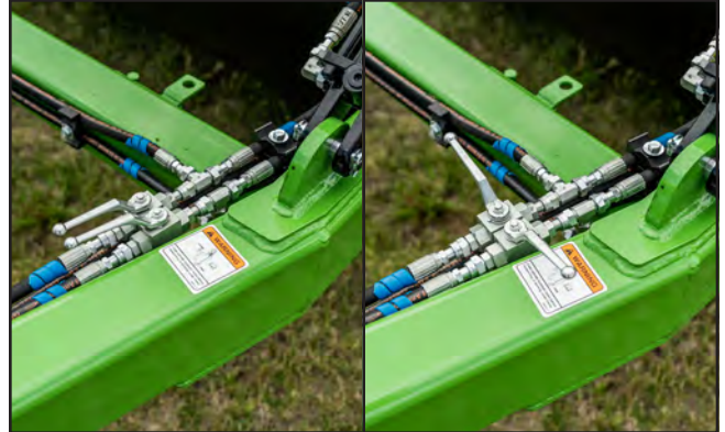
Fig. 57 Hitch Circuit Hydraulic Ball Valves: Open/Closed
