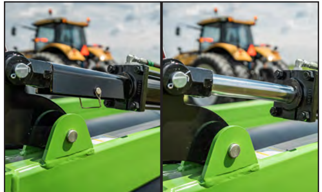
Fig. 44 Wing Cylinder Stop: Installed/Removed
