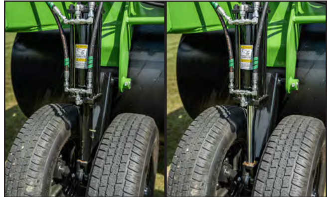
Fig. 43 Center Section Cylinder Stop: Installed/Removed
