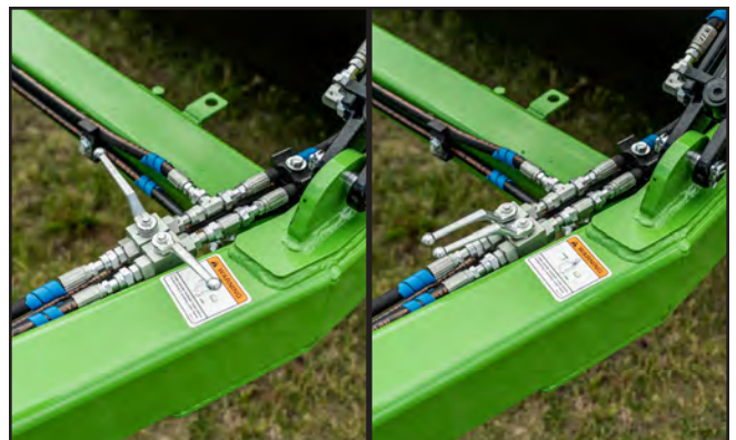
Fig. 46 Hitch Circuit Hydraulic Ball Valves: Closed/Open
