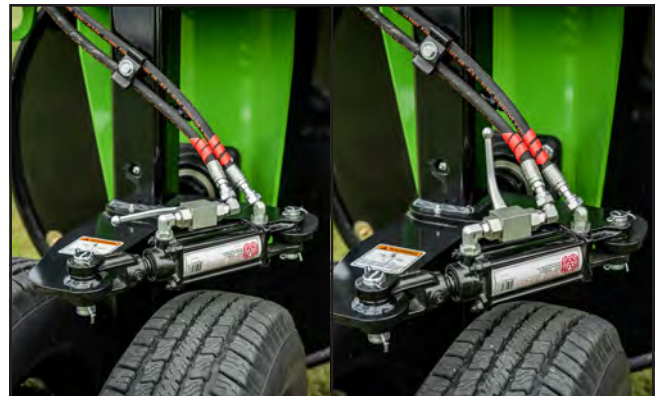
Fig. 59 Steering Circuit Hydraulic Ball Valves: Open/Closed
