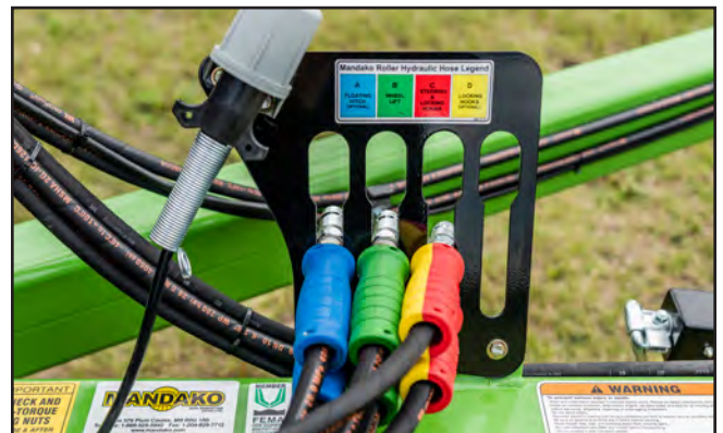
Fig. 12 Hydraulic Circuit Legend
