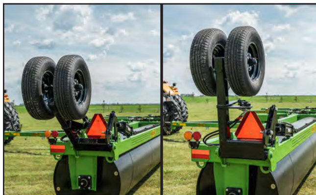
Fig. 52 Wheel Assmeblies: Raising/Raised
