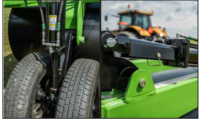
Fig. 41 Cylinder Stops Installed
