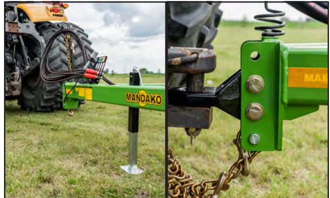
Fig. 36 Hitch Height: Jack/Pintle Mount
