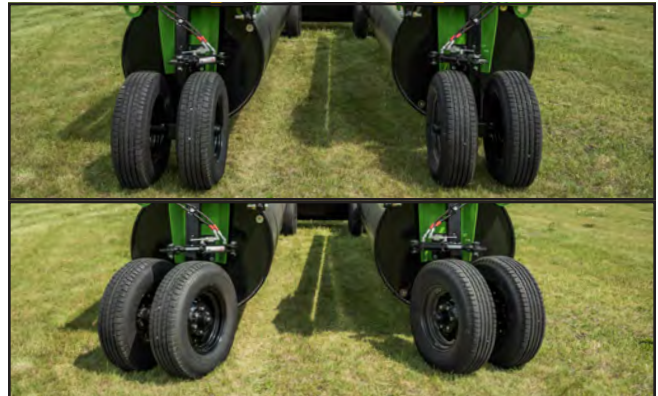
Fig. 48 Steerable Wheels: Straight/Turned
