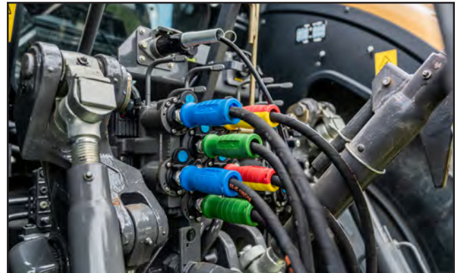
Fig. 25 Hydraulic Circuits Installed
