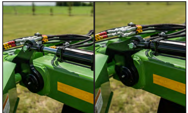
Fig. 40 Wing Lock Hooks: Engaged/Disengaged
