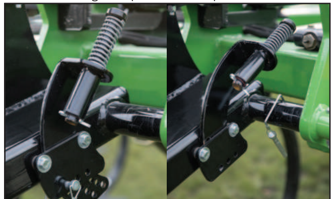
Fig. 4 Depth Control Mechanism: Working/Raised
