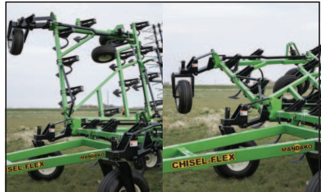
Fig. 42 Lower Wing: Starting/Almost Down
