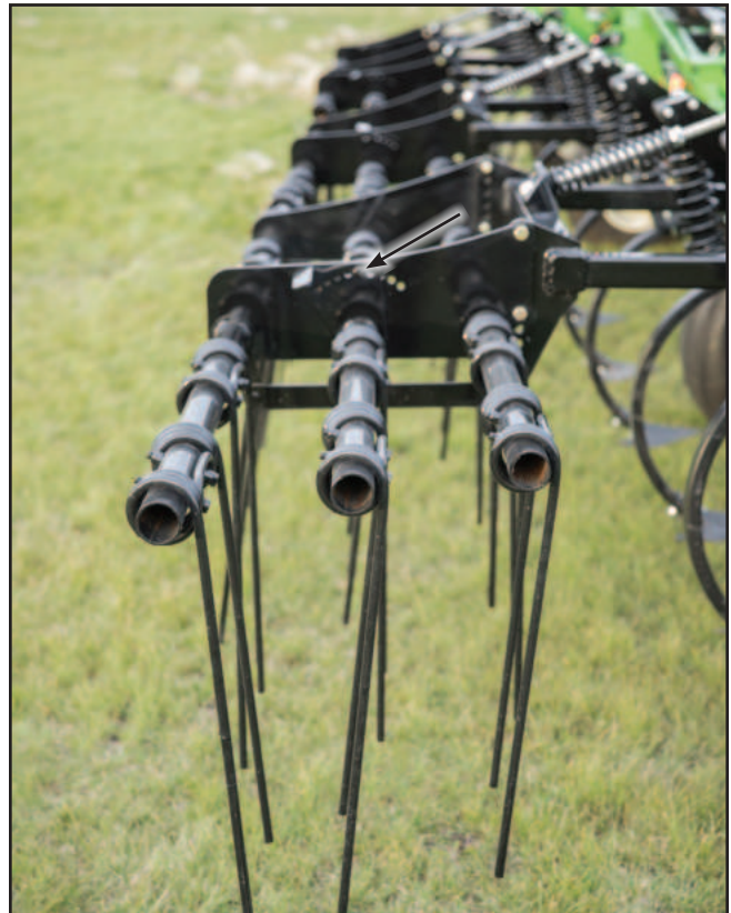
Fig. 36 Tine Harrows: Adjustment Angle
