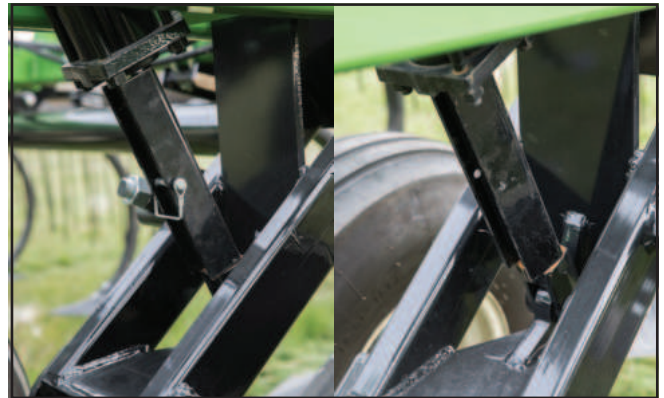
Fig. 38 Cylinder Stop: Pinned/Pin Removed
