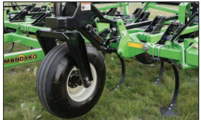
Fig. 33 Single Point Depth Control System
