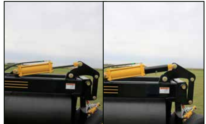
Fig. 63 Wing Section Cylinder Stop: Removed/Installed
