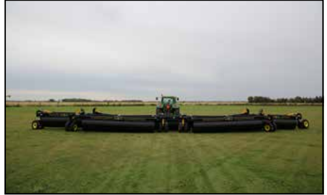
Fig. 50 Roller Drums at right angles from the direction of travel
