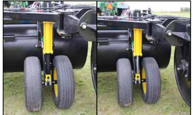
Fig. 42 Center Section Cylinder Stop: Installed/Removed
