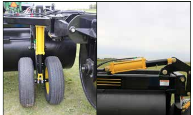
Fig. 40 Cylinder Stops Installed
