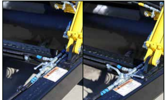
Fig. 58 Hitch Circuit Hydraulic Ball Valves: Open/Closed
