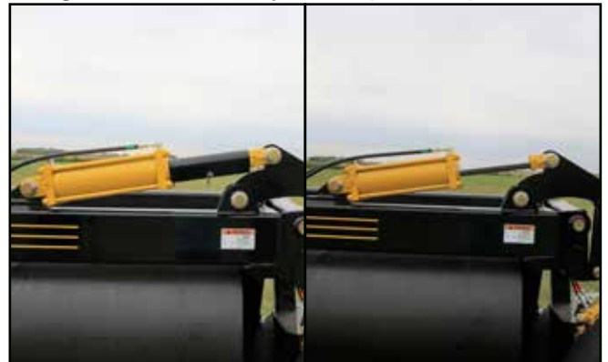
Fig. 43 Wing Cylinder Stop: Installed/Removed
