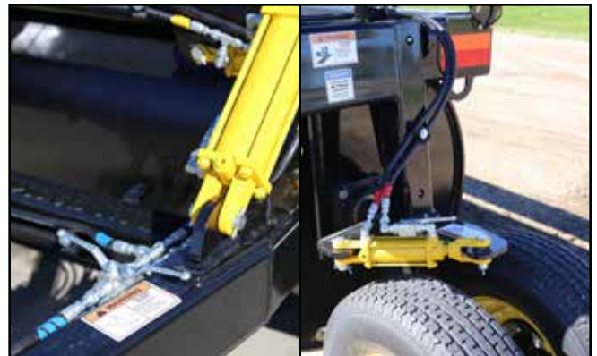
Fig. 41 Hydraulic Ball Valves: Hitch, Steering
