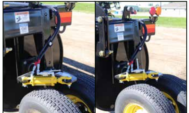
Fig. 59 Steering Circuit Hydraulic Ball Valves: Open/Closed
