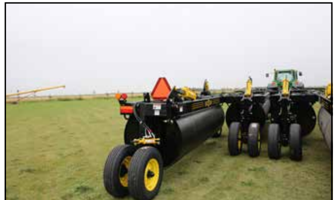
Fig. 67 Lights and SMV in place and clear to see
