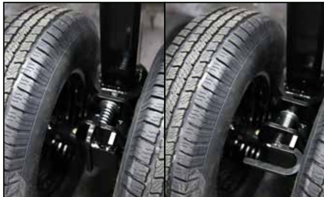
Fig. 49 Swivel Axle locks: Locked/Unlocked
