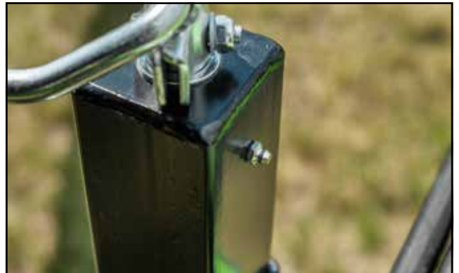
Fig. 80 Grease Hitch Jack
