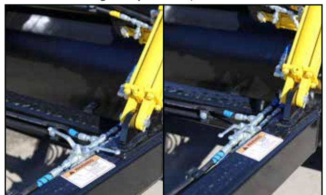
Fig. 45 Hitch Circuit Hydraulic Ball Valves: Closed/Open
