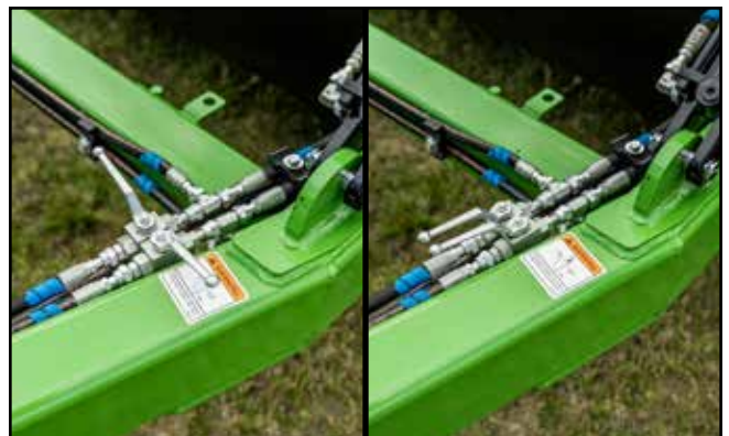
Fig. 46 Hitch Circuit Hydraulic Ball Valves: Closed/Open
