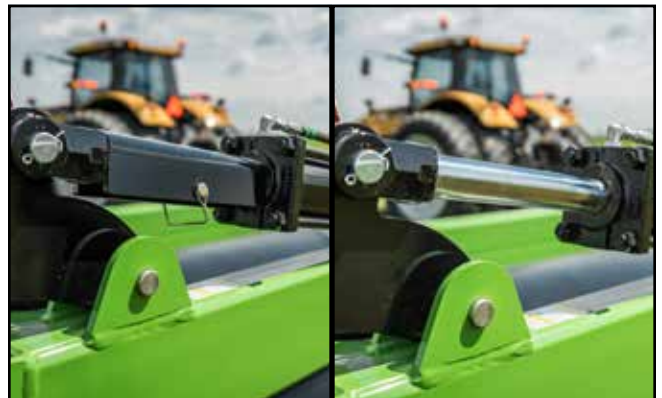
Fig. 44 Wing Cylinder Stop: Installed/Removed
