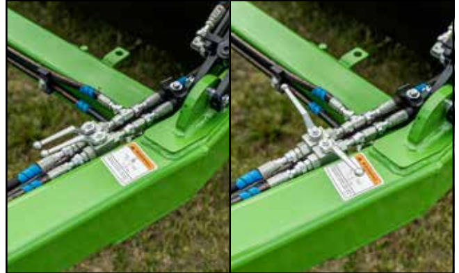
Fig. 57 Hitch Circuit Hydraulic Ball Valves: Open/Closed
