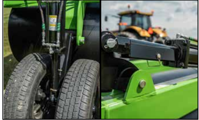
Fig. 41 Cylinder Stops Installed
