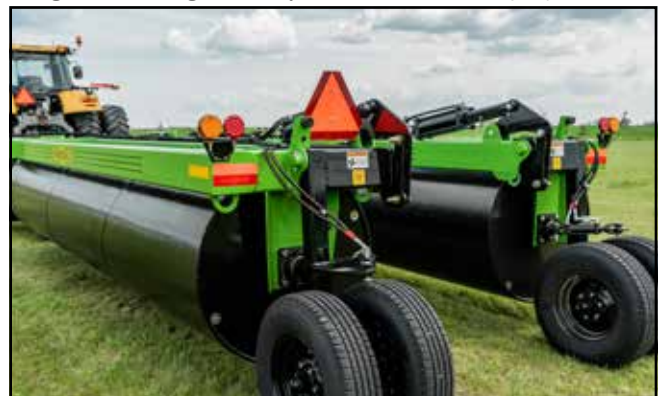
Fig. 60 Lights and SMV in place and clear to see
