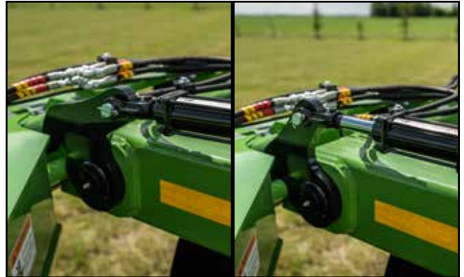
Fig. 51 Wing Lock Hooks: Disengaged/Engaged
