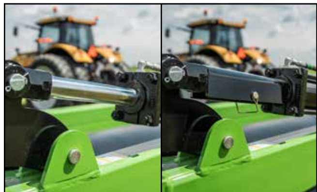
Fig. 56 Wing Section Cylinder Stop: Removed/Installed
