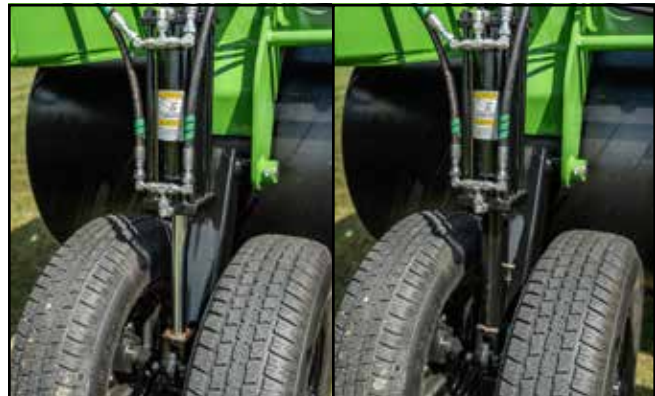
Fig. 55 Center Section Cylinder Stop: Removed/Installed
