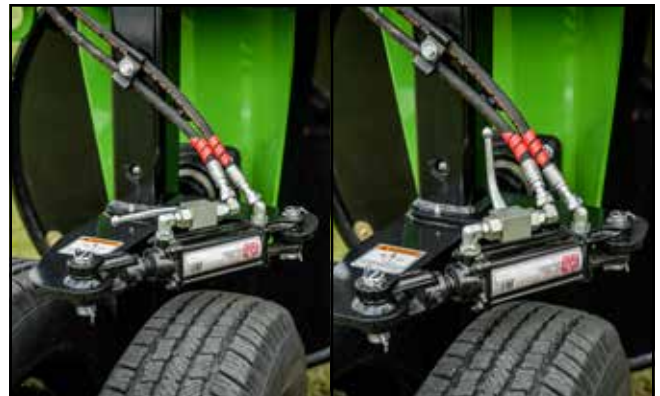
Fig. 59 Steering Circuit Hydraulic Ball Valves: Open/Closed
