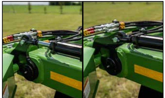
Fig. 40 Wing Lock Hooks: Engaged/Disengaged
