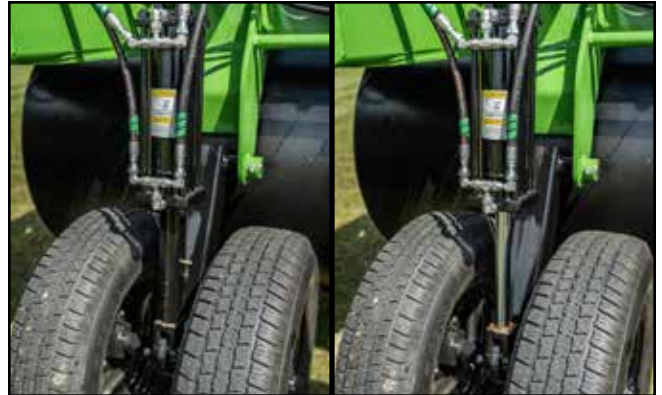
Fig. 43 Center Section Cylinder Stop: Installed/Removed
