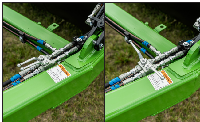
Fig. 46 Hydraulic Ball Valves: Open/Closed
