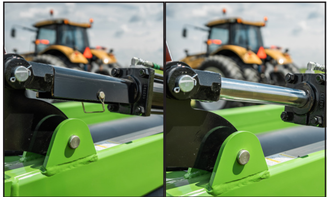
Fig. 23 Wing Cylinder Stop - Installed/Removed
