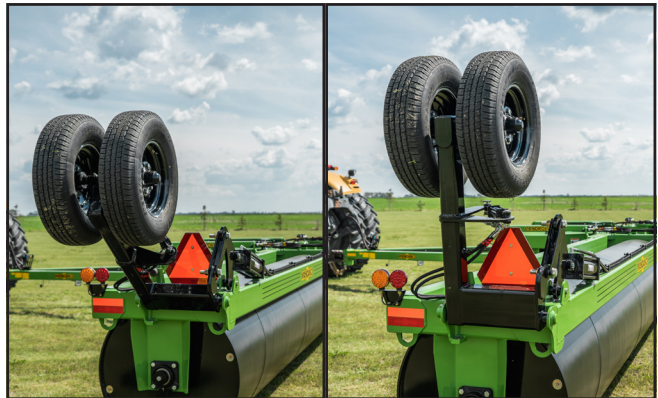
Fig. 31 Wheel Assemblies - Raising/Raised
