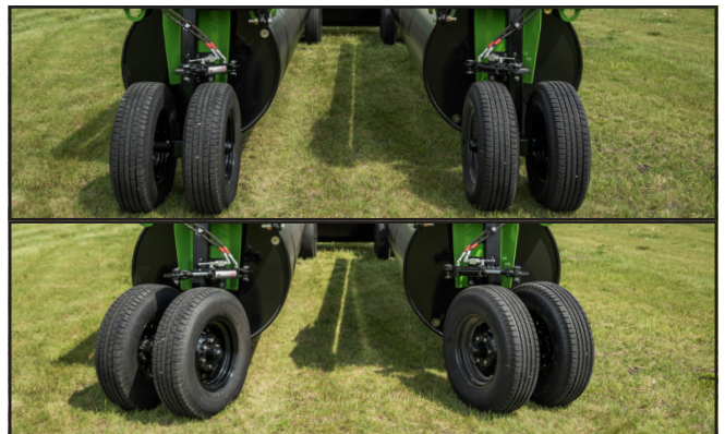
Fig. 27 Steerable Wheel Axles - Straight/Turned
