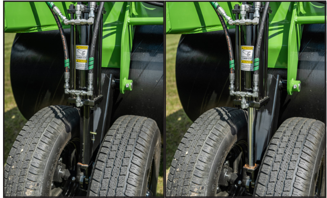
Fig. 22 Center Section Cylinder Stop - Installed/Removed
